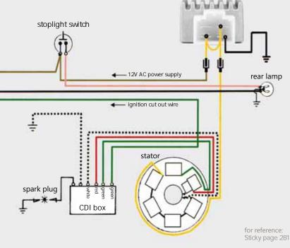
Original type AC loom, 12 V electronic ignition
