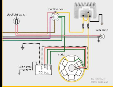
Original type DC loom, 12 V electronic ignition
