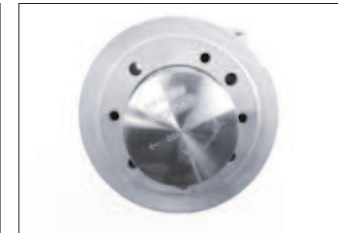
Use the piston to get the ring into square position to take accurate measurements
