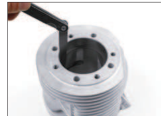
Use the feeler gauge to measure the ring gap
